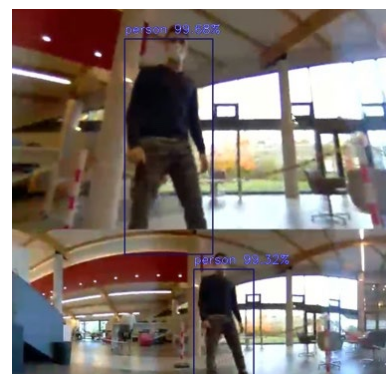
Figure 6. Use of MA to inspect for intruders onsite
