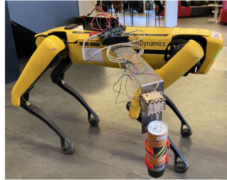
Figure 11. Use of Spot® Robot to do marking onsite
